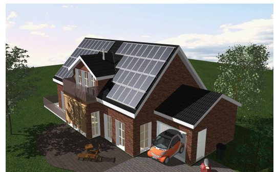
As part of the Solar Simulation in DDS-CAD PV , shading is realistically represented from shading objects.
